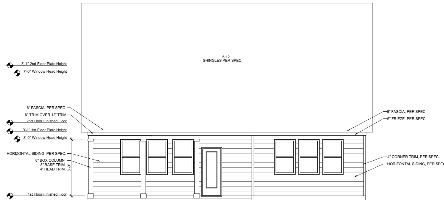
BIRCH II REAR ELEVATION SCALE: 1/8"=1'-0" (11"X17" SHEET SIZE) SCALE: 1/4"=1'-0" (22"X34" SHEET SIZE)
