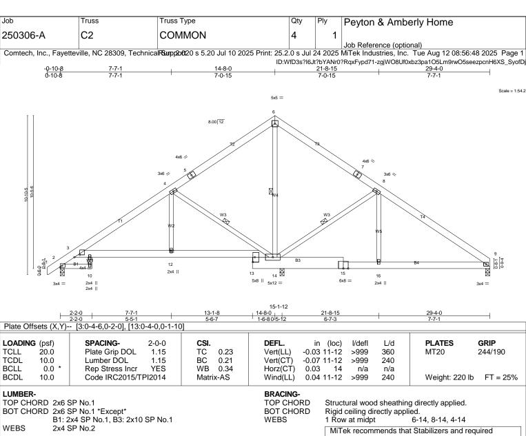
cross bracing be installed during truss erection, in accordance with Stabilizer Installation guide.
