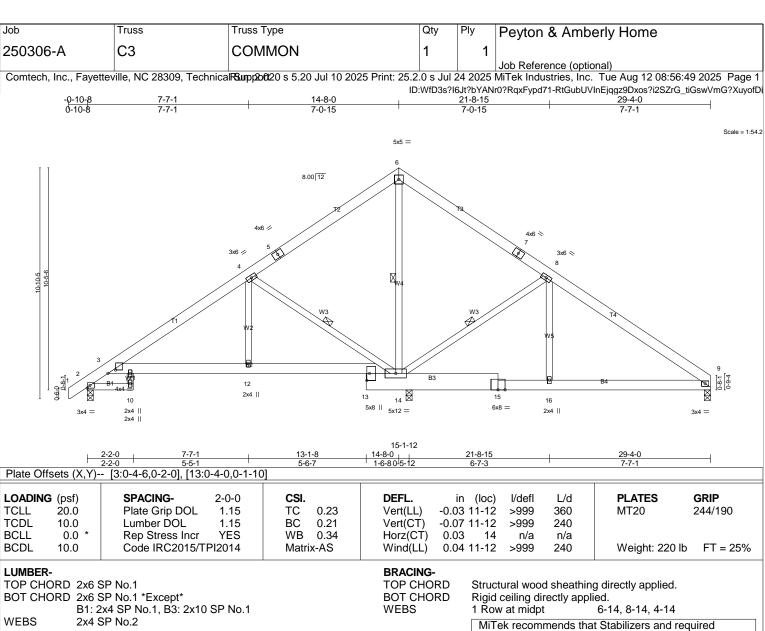
MiTek recommends that Stabilizers and required cross bracing be installed during truss erection, in accordance with Stabilizer Installation guide.
