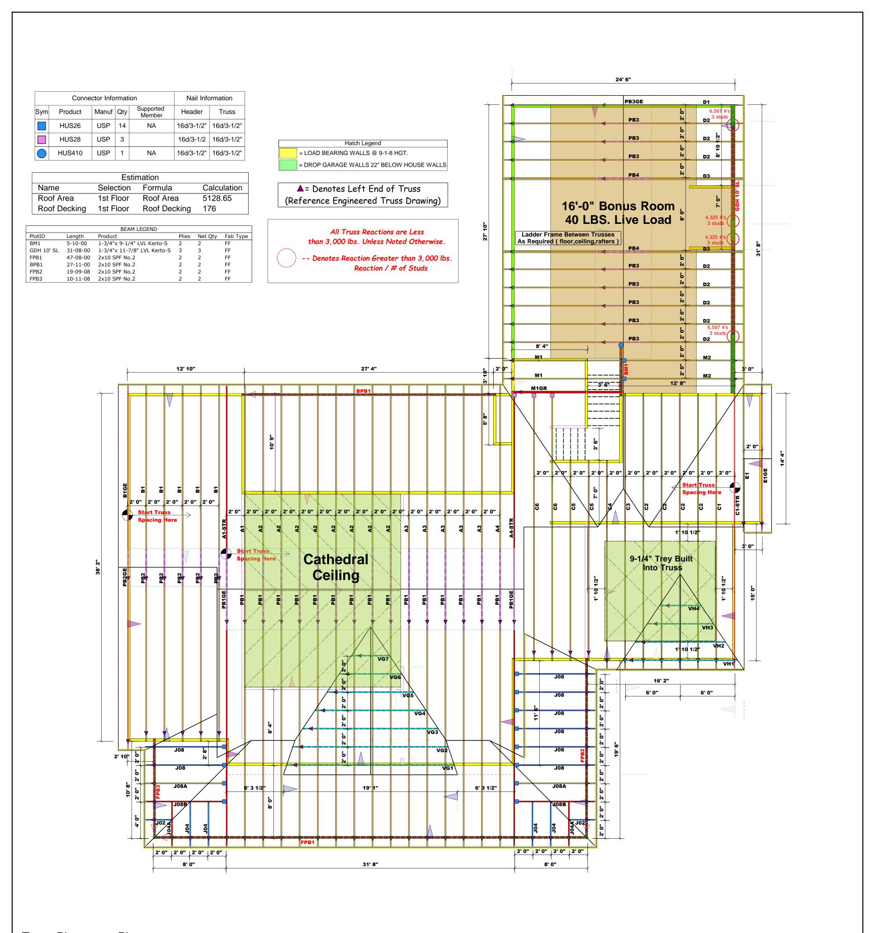
Truss Placement Plan
