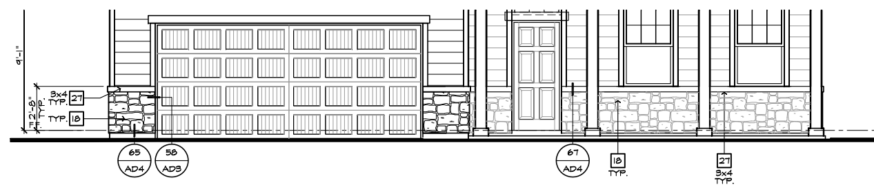
PARTIAL FRONT ELEVATION 'D' W/ MASONRY OPTION AT 9'-0" PLT. HGT. SCALE 1/4"=1'-0" (22'x34") - 1/8"=1'-0" (11'x17")
