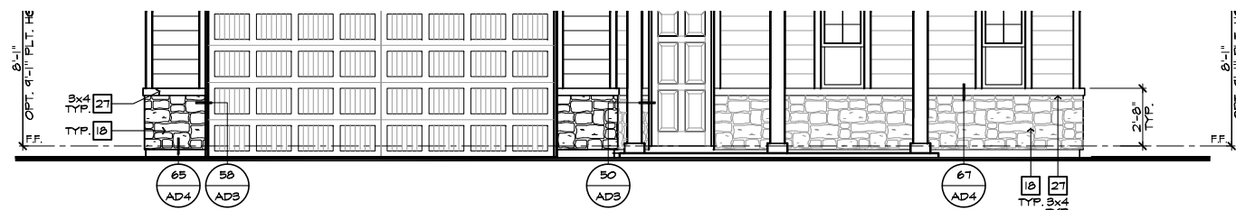
PARTIAL FRONT ELEVATION 'C' W/ MASONRY OPTION
