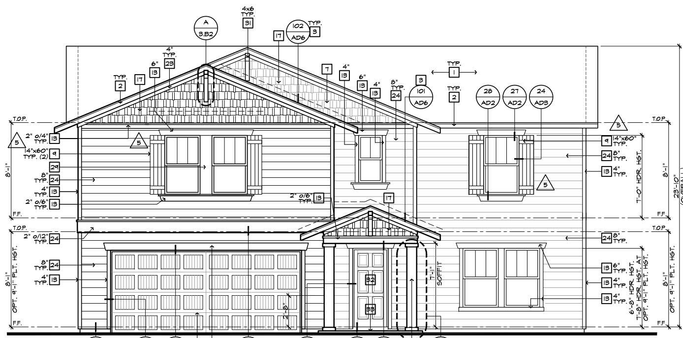
REAR ELEVATION 'B' SCALE 1/4"=1'-0" (22"X34") - 1/8"=1'-0" (11"X17")
