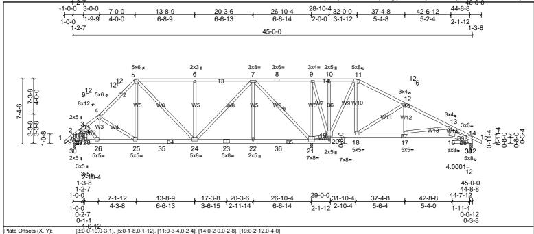
DEFL PLATES 2-0-0 CSI in I/defl L/d GRIP Loading (psf) Spacing (loc) TCLL (roof) 20.0 Plate Grip DOL 1.15 TC 0.68 Vert(LL) 0.03 16-17 >999 240 MT20 244/190 TCDL 10.0 Lumber DOL 1.15 BC 0.28 Vert(CT) -0.06 16-17 >999 180 BCLL NO WB 0.0 Rep Stress Incr Horz(CT) 0.02 0.81 14 n/a n/a BCDI 10.0 Code IRC2015/TPI2014 Matrix-MSH Weight: 347 lb FT = 20%
