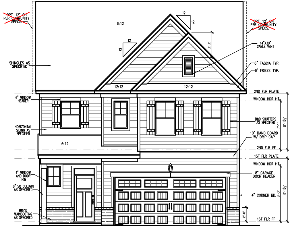
FRONT DOOR STYLE PER PURCHASE ORDER FRONT ELEVATION 'A' SCALE: 1/4" = 1'-0" ON 22x34, 1/8" = 1'-0" ON 11x17
