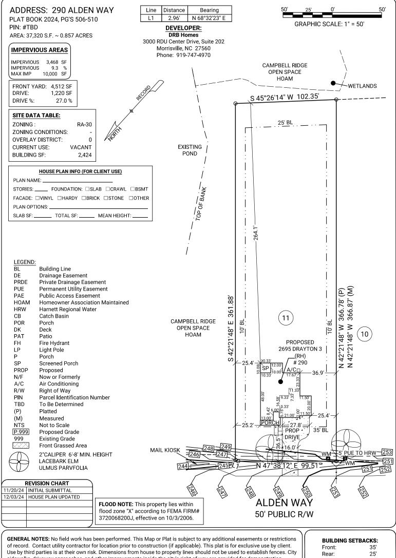
sidewalks, driveway approaches, and other improvements inside the city's right of way are provided for demonstration purposes only. consult the development plans for actual construction. This plat has been calculated for closure and is found to be accurate within one foot in 10,000+ feet.
