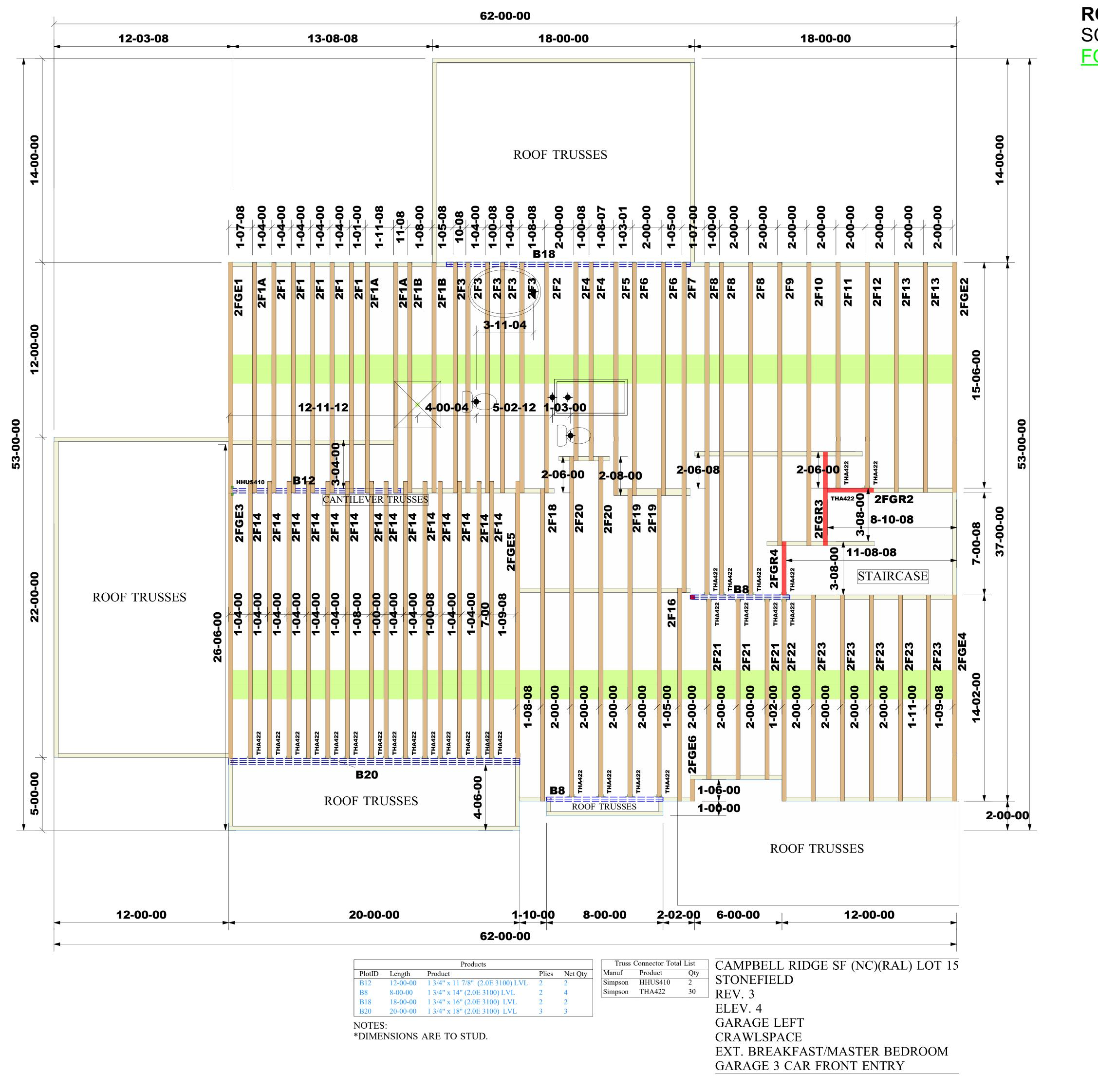
ROOF TRUSS LAYOUT SCALE: NTS
