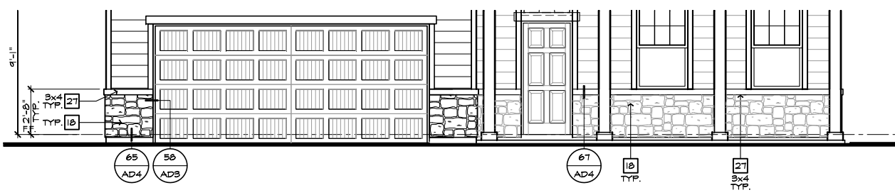
PARTIAL FRONT ELEVATION 'D' W/ MASONRY OPTION AT 9'-0" PLT. HGT. SCALE 1/4"=1'-0" (22'x34") - 1/8"=1'-0" (11'x17")
