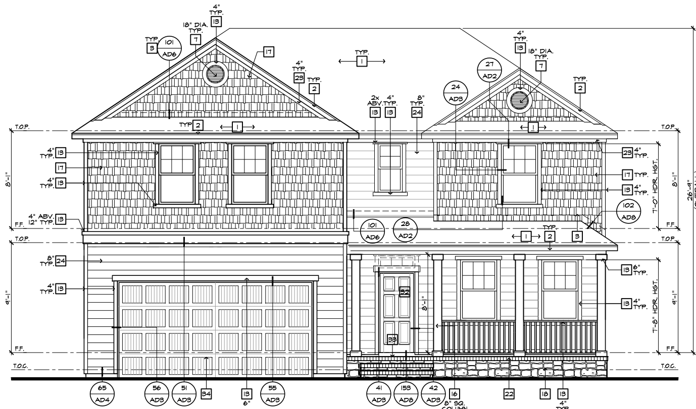
FRONT ELEVATION 'D' W/ CRAWL SPACE AT OPTIONAL 9'-1" PLT. HGT. SCALE 1/4"=1'-0" (22'x34") - 1/8"=1'-0" (11'x17")
