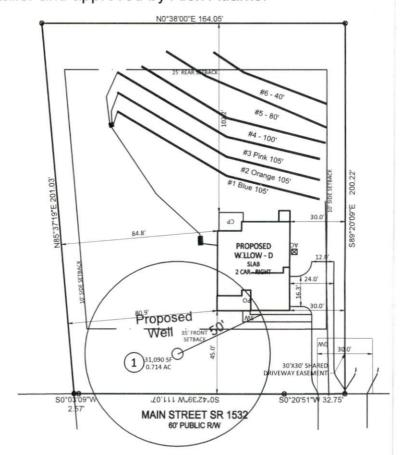
System: Gravity to D-Box Lines: 1-3 (315') 0.4 LTAR 24" Max Trench Bottom Accepted Status System Repair: Pressure Manifold Lines: 4-6 (220') 0.4LTAR 24" Max Trench Bottom
