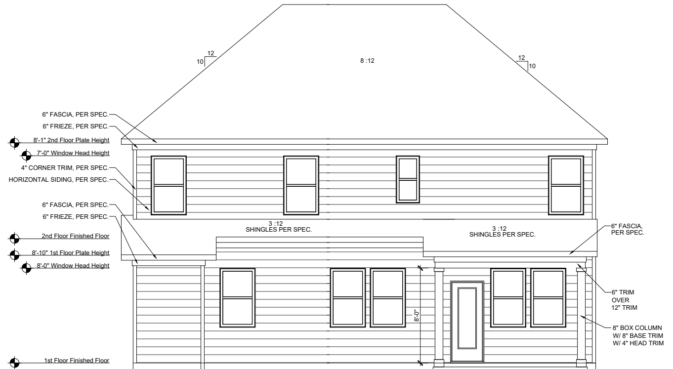
WELL HOUSE ADDITION REAR ELEVATION SCALE: 1/8"=1'-0" (11"X17" SHEET SIZE) SCALE: 1/4"=1'-0" (22"X34" SHEET SIZE)
