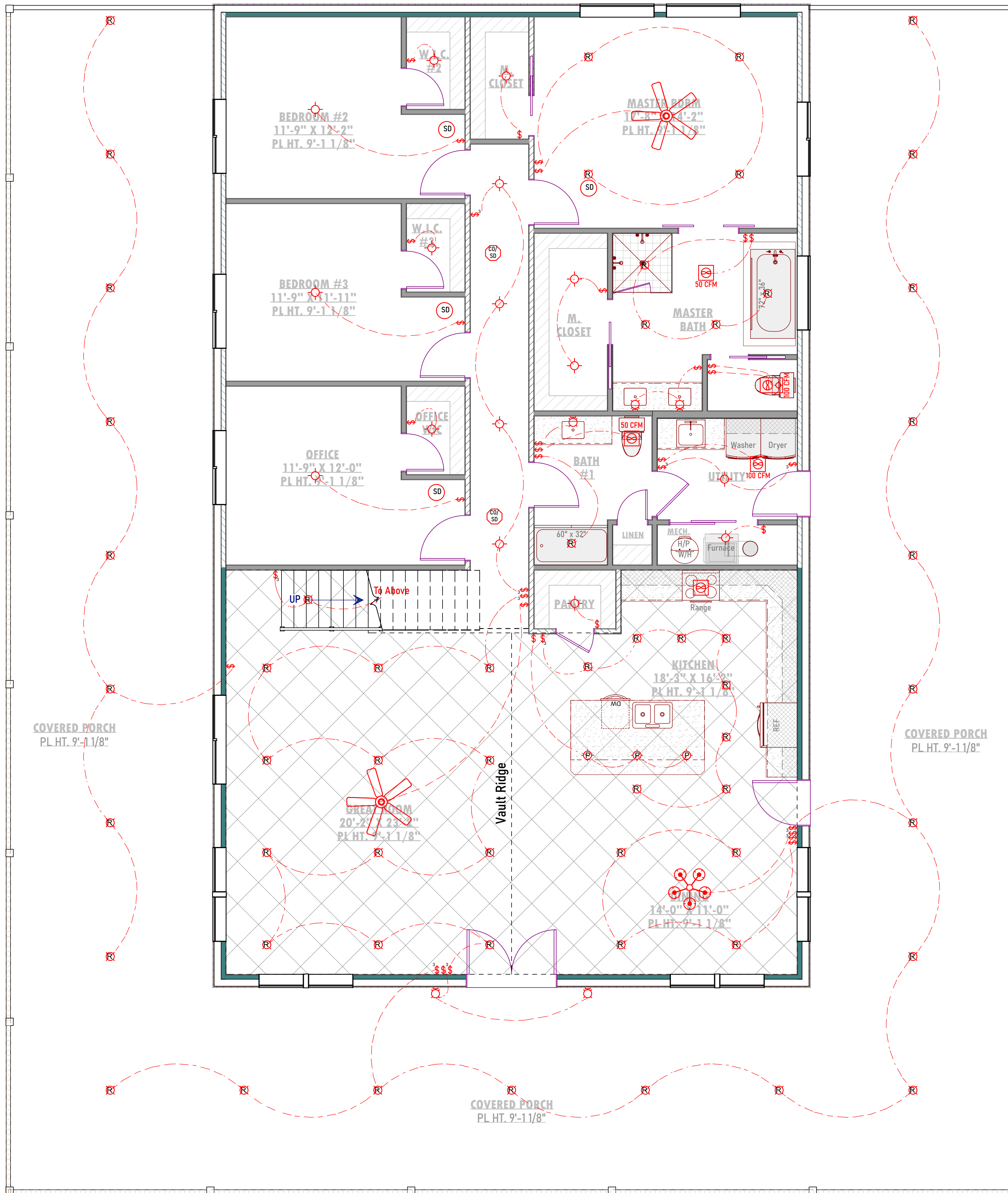
1ST FLOOR PROPOSED LIGHTING PLAN Scale - 1/4" = 1'-0"
