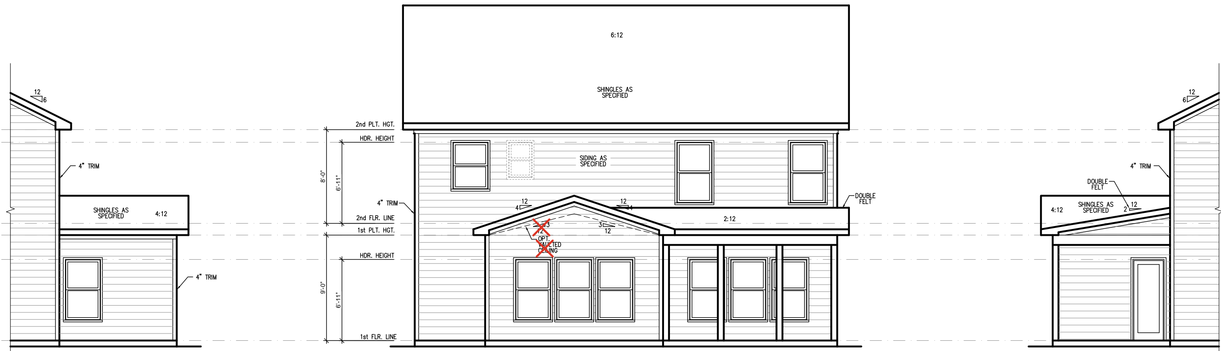
EXTENDED CAFE W/ COVERED PORCH REAR ELEVATION SCALE: 1/8"=1'-0" ON 11x17, 1/4"=1'-0" ON 22x34
