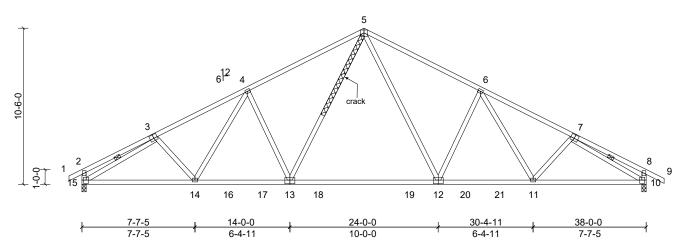
Repair for a crack in the web where indicated.
