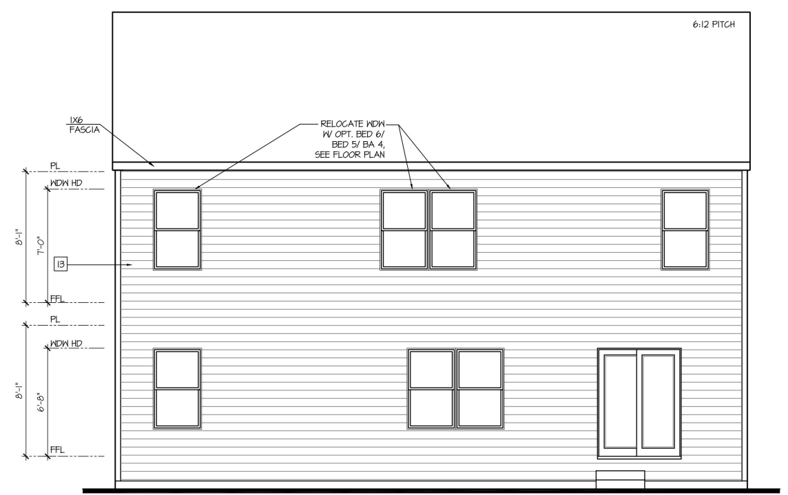
Rear Elevation 'F' w/ Opt Crawl Space SCALE: 1/4"=1'-0" AT 22'X34" LAYOUT 1/8"=1'-0" AT 11'X11" LAYOUT
