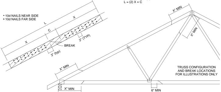
HE LOCATION OF THE BREAK MUST BE GREATER THAN OR EQUAL TO THE REQUIRED X DIMENSION FROM ANY PERIMETER BREAK OR HEEL JOINT AND A MINIMUM OF 6" FROM ANY INTERIOR JOINT (SEE SKETCH ABOVE)
