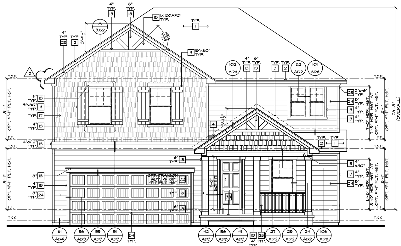
FRONT ELEVATION 'C' W/ CRAWL SPACE SCALE 1/4"=1'-0" (22"x34") - 1/8"=1'-0" (11"x17")
