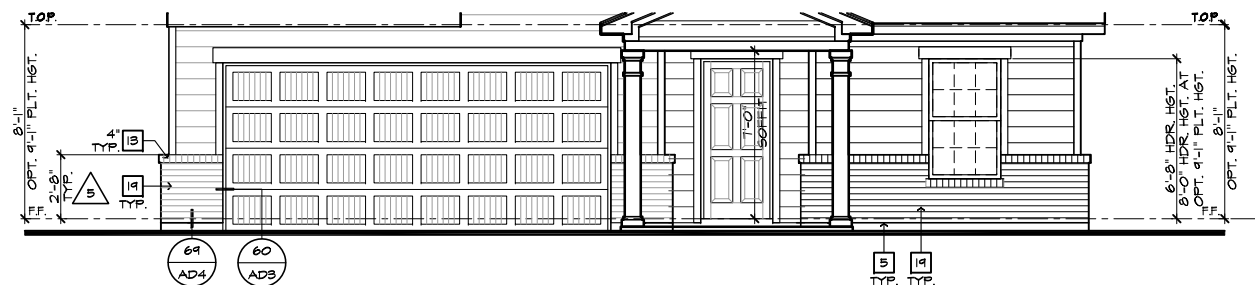
PARTIAL FRONT ELEVATION 'A' W/ BRICK OPTION
