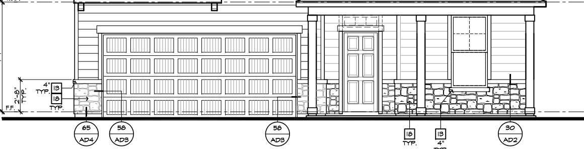
PARTIAL FRONT ELEVATION 'D' AT OPTIONAL 9'-1" PLT. HGT. W/ STONE OPT.
