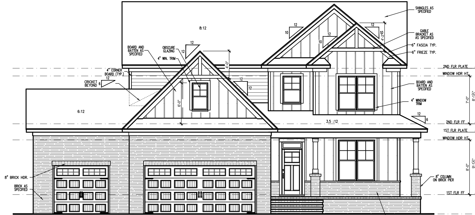
FRONT ELEVATION 'E' - 3 CAR FRONT LOAD (CRAWL)
