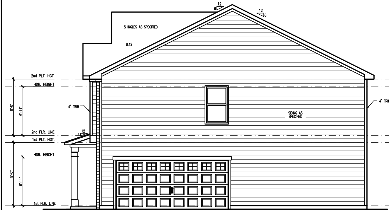
OPT. 2-CAR SIDELOAD GARAGE RIGHT SIDE ELEVATION 'GEORGIAN' (SLAB) SCALE: 1/4" = 1'-0" ON 22x34, 1/8" = 1'-0" ON 11x17
