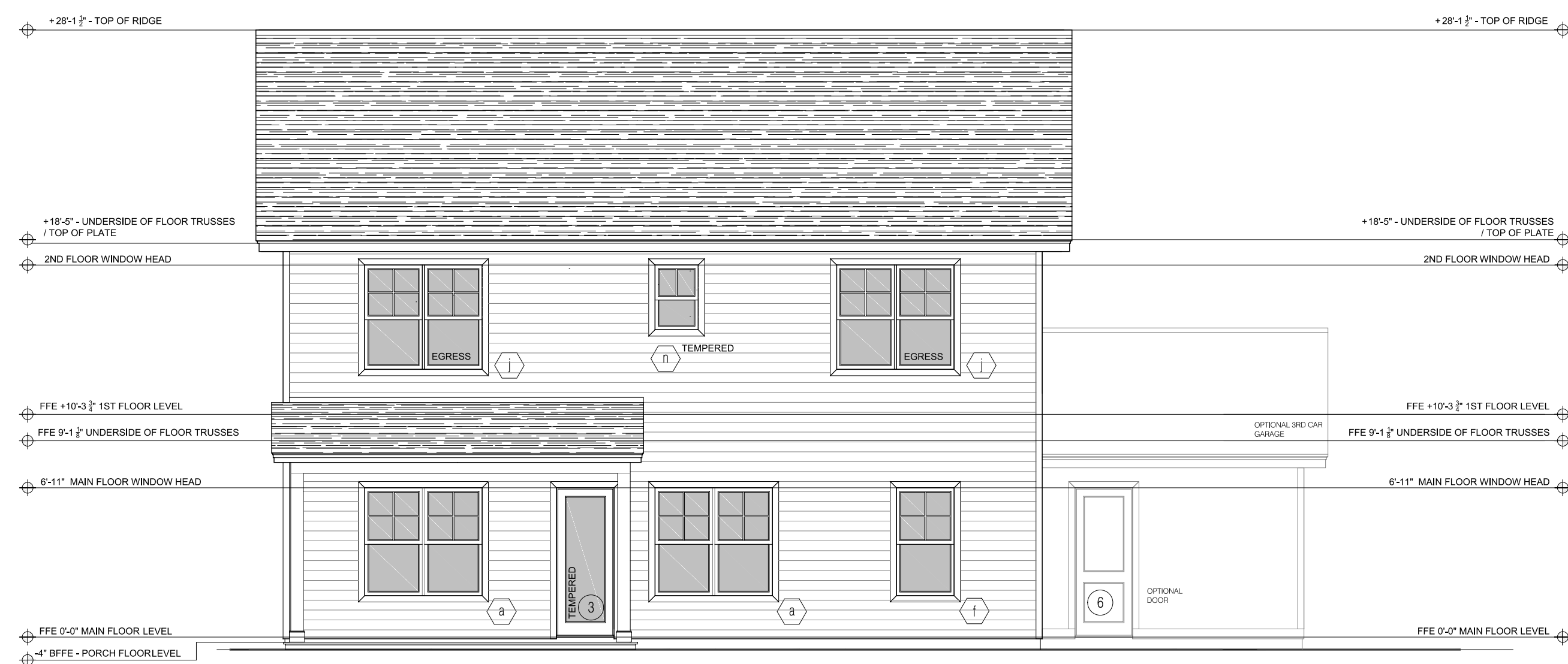
REAR ELEVATION SCALE: 1/4" = 1'-0"
