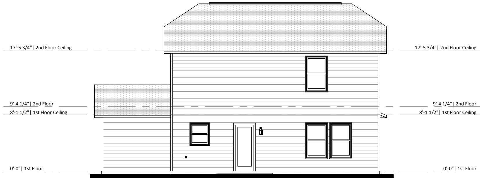
② Rear Elevation - Elev B - 2 Car Garage 1/8" = 1'-0"
