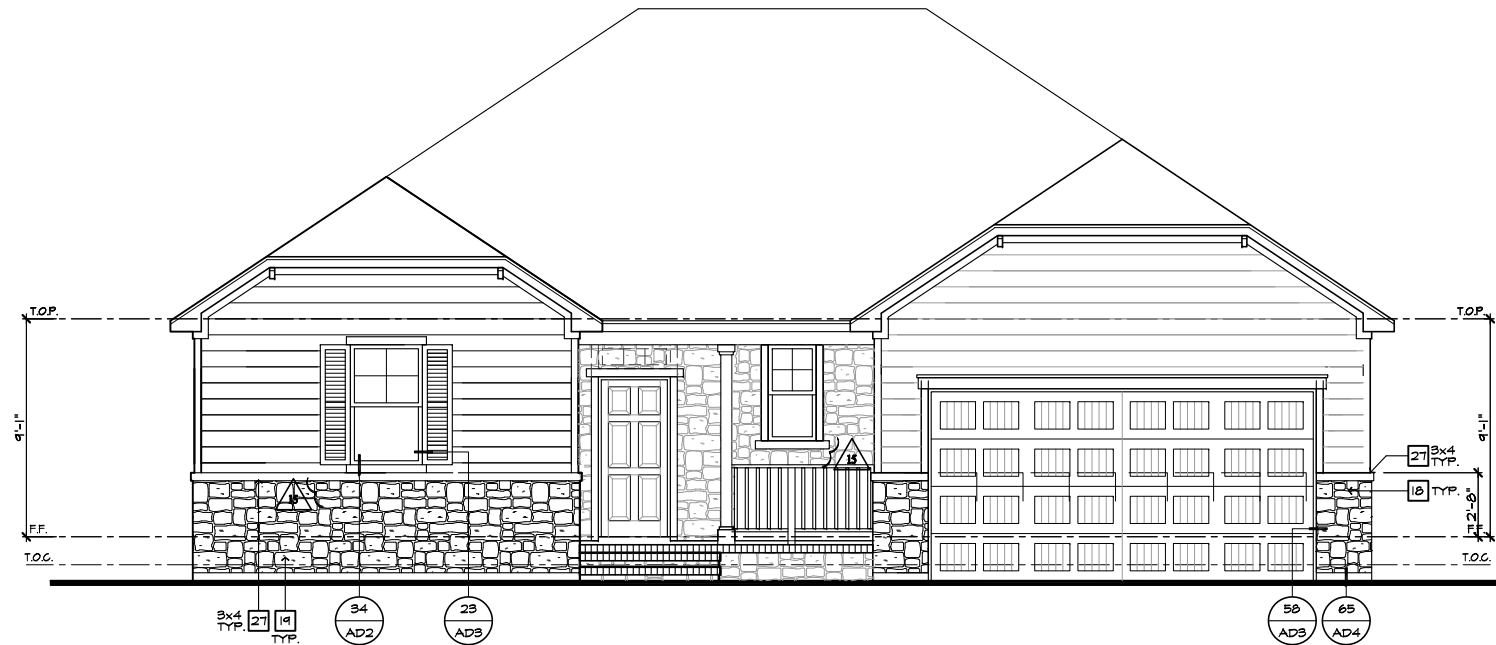
FRONT ELEVATION 'D' W/ STONE AT CRAWL SPACE AT OPTIONAL 9'-1" PLT. HGT.
