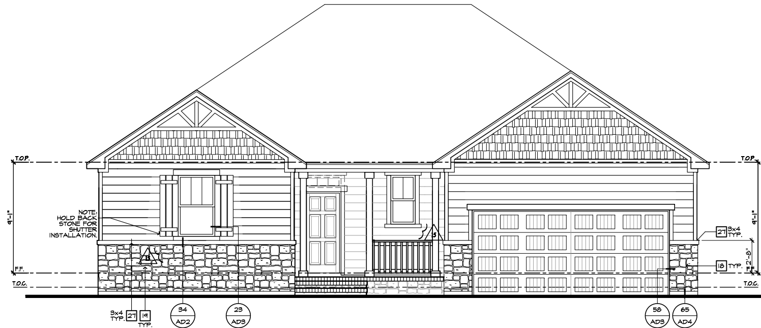
FRONT ELEVATION 'C' W/ STONE AT CRAWL SPACE AT OPTIONAL 9'-1" PLT. HGT.
