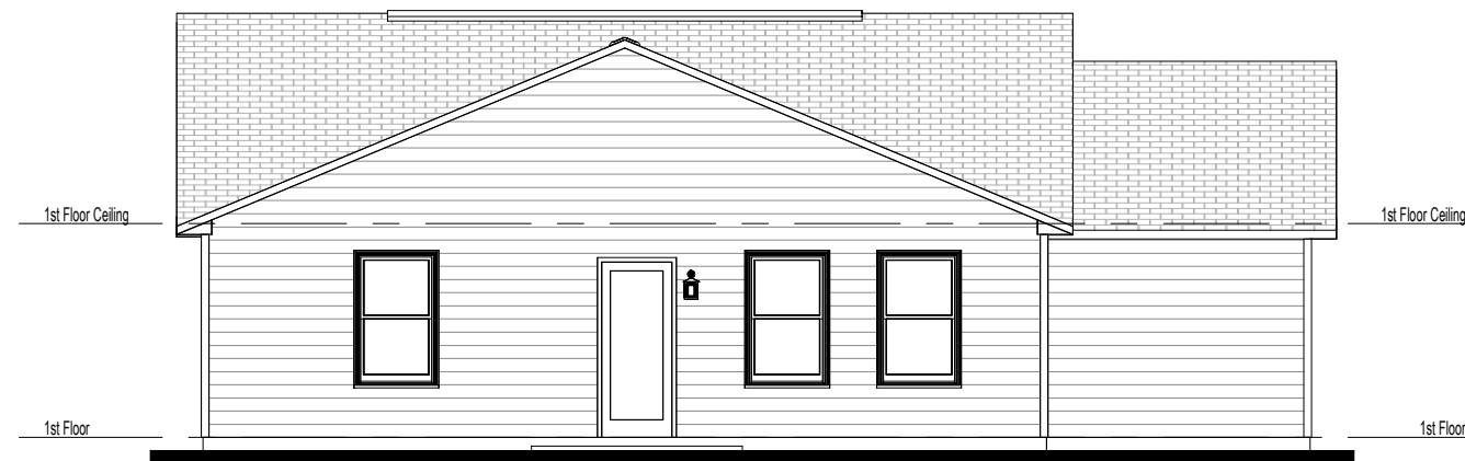
2 Rear Elevation - Elev A - 2 Car Garage 1/8" = 1'-0"
