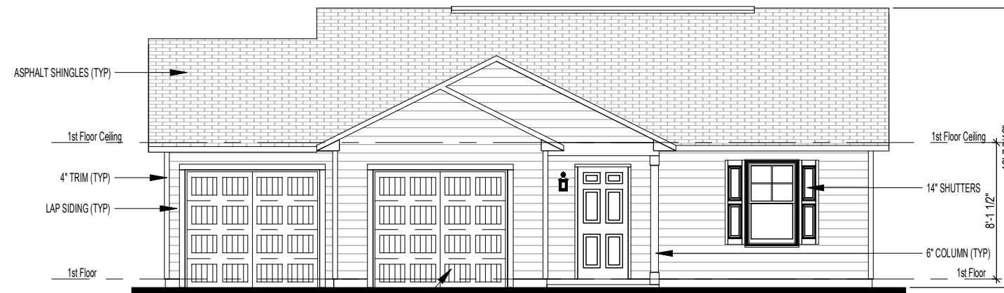
1 Front Elevation - Elev A - 2 Car Garage 1/8" = 1'-0"
