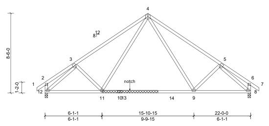
Repair for a 6" wide by 1" deep semi-circular notch in the top edge of the bottom chord where indicated.
