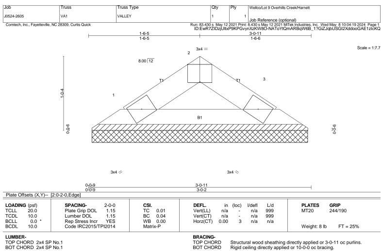
MiTek recommends that Stabilizers and required cross bracing be installed during truss erection, in accordance with Stabilizer Installation guide.
