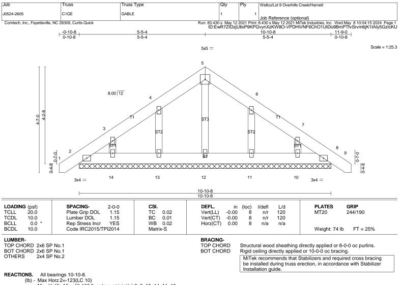
Max Uplift All uplift 100 lb or less at joint(s) 2, 8, 13, 14, 11, 10 Max Grav All reactions 250 lb or less at joint(s) 2, 8, 12, 13, 14, 11, 10
