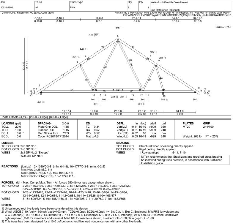
4) \* This truss has been designed for a live load of 30.0psf on the bottom chord in all areas where a rectangle 3-6-0 tall by 2-0-0 wide will fit between the bottom chord and any other members, with BCDL = 10.0psf.
