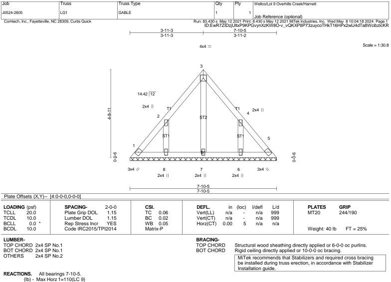
Max Uplift All uplift 100 lb or less at joint(s) 1, 5 except 8=-128(LC 12), 6=-127(LC 13) Max Grav All reactions 250 lb or less at joint(s) 1, 5, 7, 8, 6
