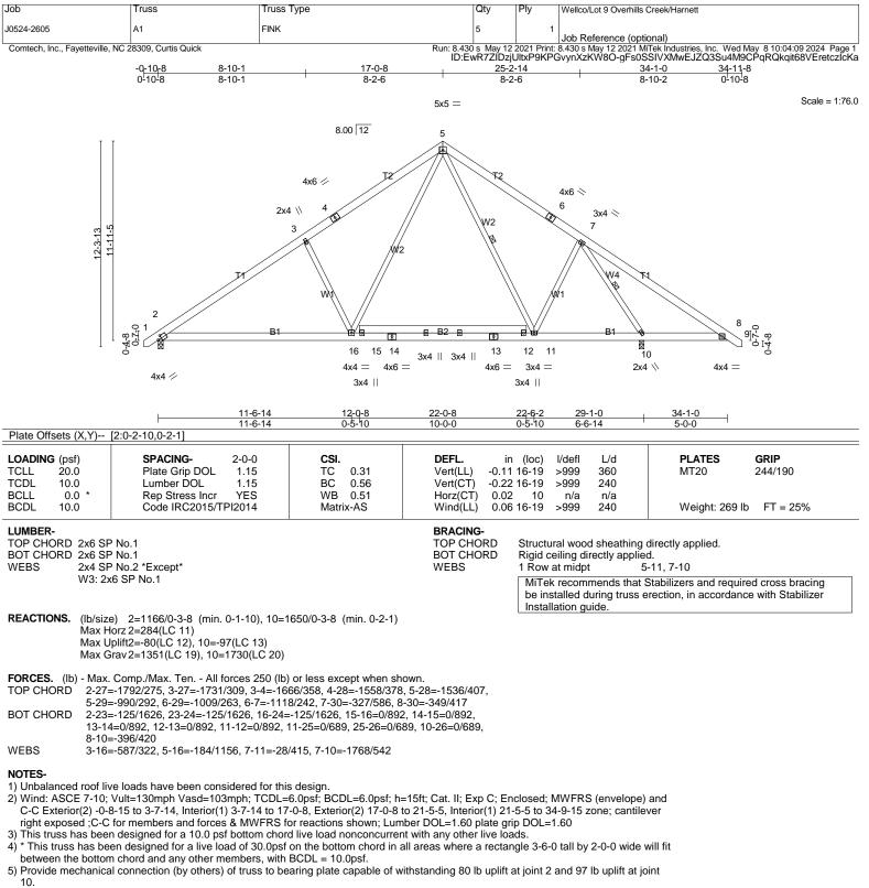
6) This truss is designed in accordance with the 2015 International Residential Code sections R502.11.1 and R802.10.2 and referenced standard ANSI/TPI 1.
