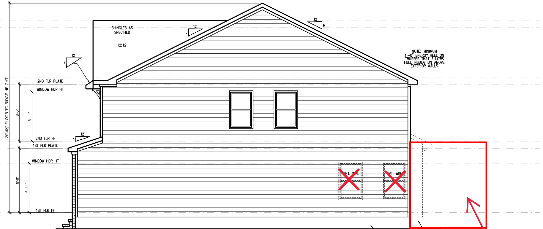
RIGHT SIDE ELEVATION 'ENGLISH COUNTRY' (CRAWL/ STEM WALL) SCALE: 1/4" = 1'-0" ON 22x34, 1/8" = 1'-0" ON 11x17 *SEE FOUNDATION PAGES FOR FOUNDATION TYPE
