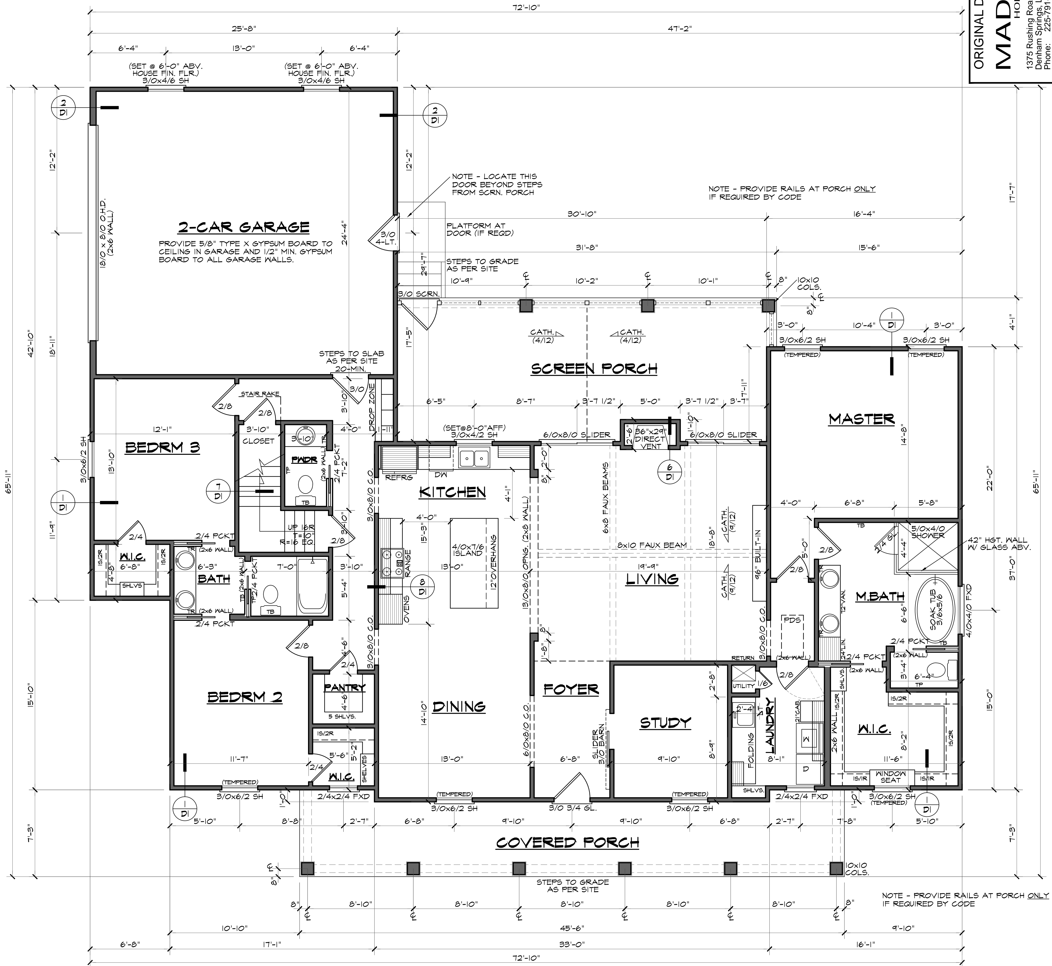
FIRST FLOOR PLAN SCALE: 1/4"=1'-0" 9'-0" CLG. HGT. U.N.O. SET WINDOWS @ 7'-4" U.N.O.
