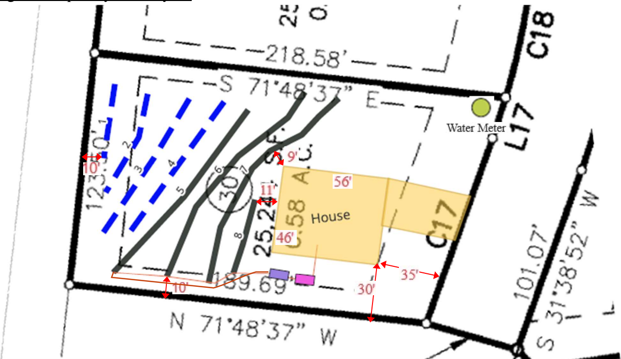
Figure 2 Septic System Layout
