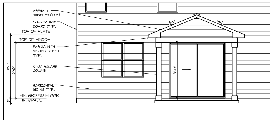
COVERED VERANDA PPO - REAR ELEVATION
