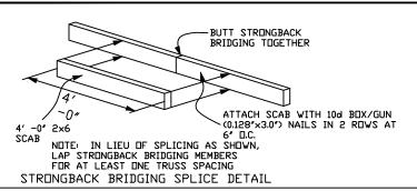
NDTE: Details 1 and 2 are the preferred attachment methods ATTACH STRONGBACK TO
