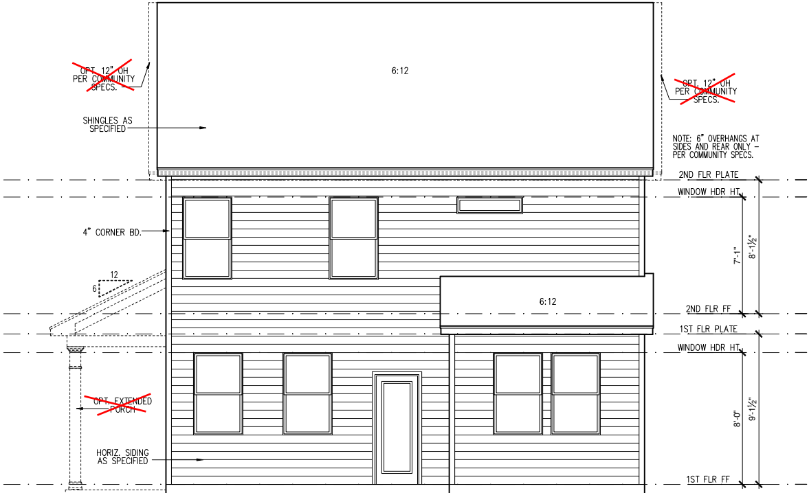
REAR ELEVATION 'A' SCALE: 1/4" = 1'-0" ON 22x34, 1/8" = 1'-0" ON 11x17
