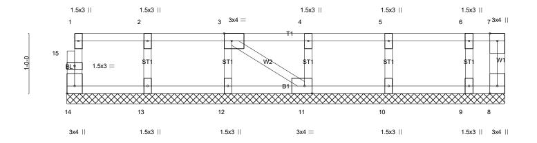
Plate Offsets (X,Y)-- [3:0-1-8,Edge], [11:0-1-8,Edge], [14:Edge,0-1-8] LOADING (psf) SPACING-CSI. DEFL PLATES **GRIP** 2-0-0 in (loc) I/defl I/d TCLL 40.0 Plate Grip DOL 1.00 TC 0.06 Vert(LL) n/a n/a 999 MT20 244/190 TCDL 10.0 Lumber DOL 1.00 вс 0.01 Vert(CT) n/a n/a 999 **BCLL** YES WB 0.03 0.00 8 0.0 Rep Stress Incr Horz(CT) n/a n/a BCDL Code IRC2021/TPI2014 Weight: 33 lb FT = 20%F, 11%E Matrix-P
