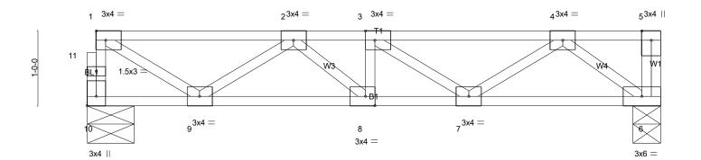
7-7-10 3-9-4 3-10-6 Plate Offsets (X,Y)-- [3:0-1-8,Edge], [8:0-1-8,Edge], [10:Edge,0-1-8] LOADING (psf) SPACING-DEFL PLATES **GRIP** 1-4-0 CSI. in (loc) I/defl L/d **TCLL** 40.0 Plate Grip DOL 1.00 TC 0.23 Vert(LL) -0.01 8 >999 480 MT20 244/190 TCDL 10.0 Lumber DOL 1.00 вс 0.23 Vert(CT) -0.03 8 >999 360 WB 0.27 0.01 6 **BCLL** 0.0 Rep Stress Incr NO Horz(CT) n/a n/a BCDL Code IRC2021/TPI2014 Weight: 40 lb FT = 20%F, 11%E Matrix-P
