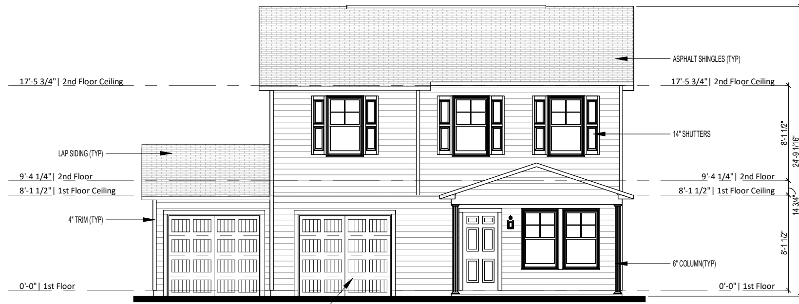
1 Front Elevation - Elev A - 2 Car Garage 1/8" = 1'-0"
