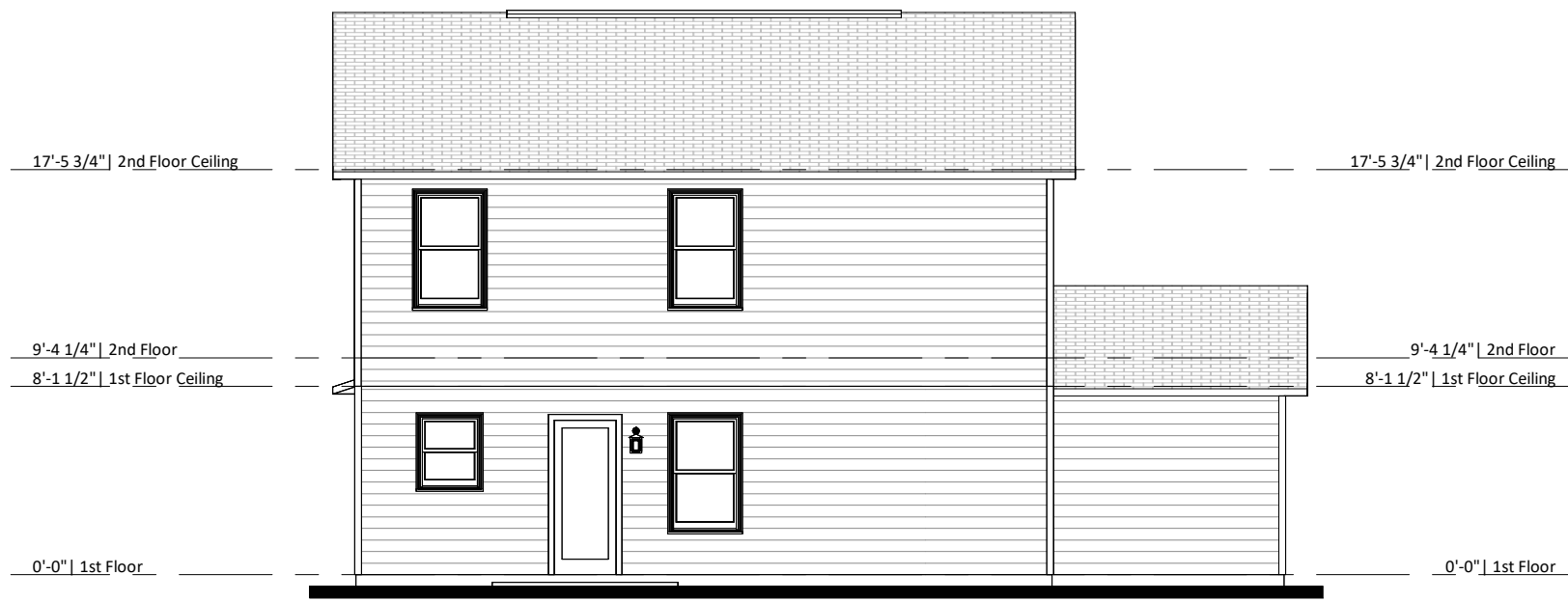
2 Rear Elevation - Elev A - 2 Car Garage 1/8" = 1'-0"
