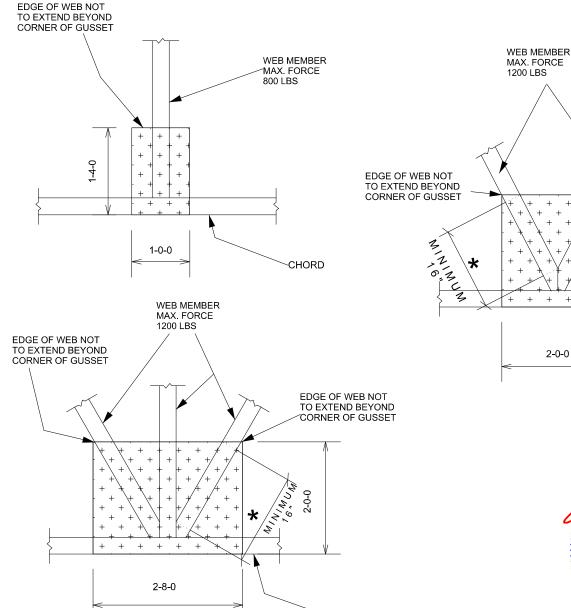
MEASUREMENT TAKEN AT POINTS WHERE WEB ACHIEVES FULL MEMBER DEPTH (AS MEASURED PERPENDICULAR TO WEB'S SAW-MILLED EDGE)
