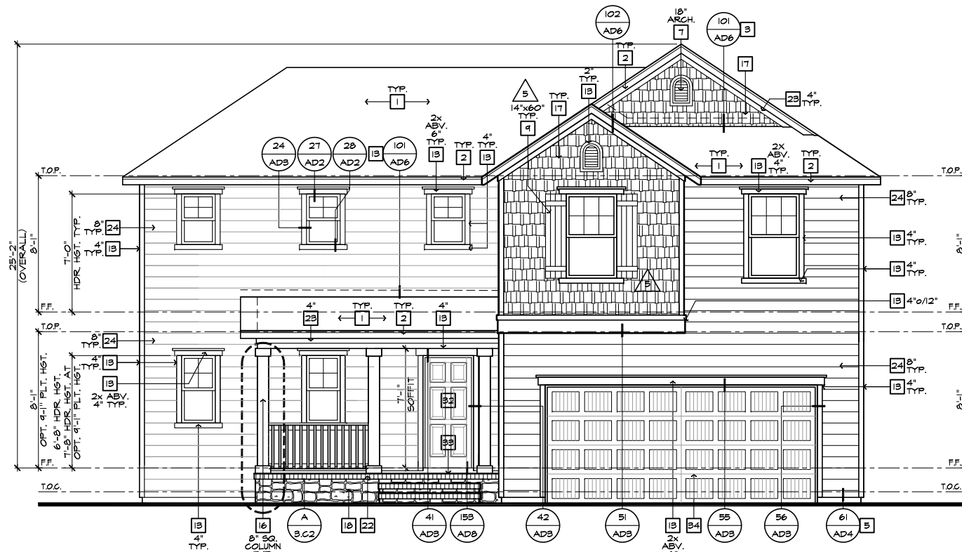
FRONT ELEVATION 'C' W/ CRAWL SPACE
