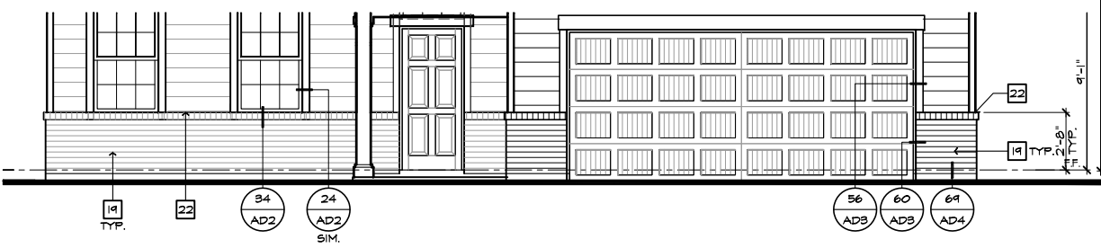
PARTIAL FRONT ELEVATION 'A' W/ MASONRY OPTION AT 9'-0" PLT. HGT. SCALE 1/4"=1'-0" (22"X34") - 1/8"=1'-0" (11"X17")
