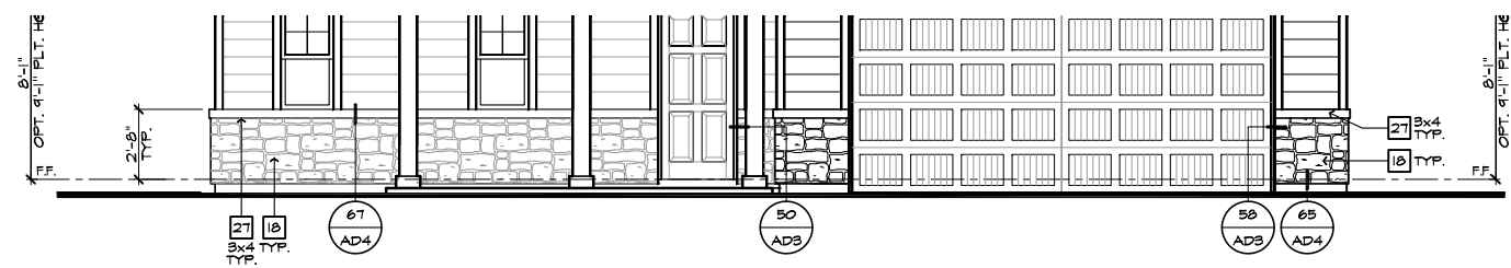
PARTIAL FRONT ELEVATION 'C' W/ MASONRY OPTION
