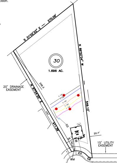
INITIAL: Lines 1-3 (300') Accepted Status Gravity Parallel REPAIR: Lines 4-5 (200') PPBPS Gravity Parallel
