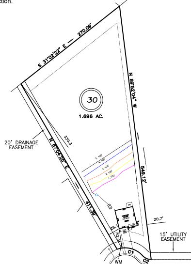
INITIAL: Lines 1-3 (300') Accepted Status Gravity Parallel REPAIR: Lines 4-5 (200') PPBPS Gravity Parallel
