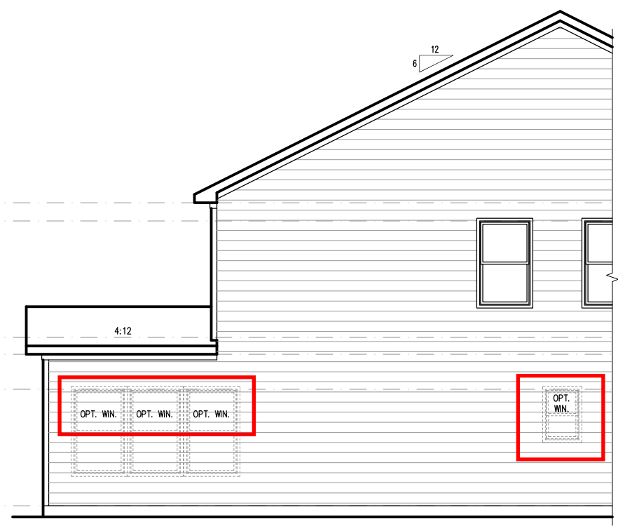
EXTENDED CAFE PARTIAL LEFT SIDE ELEVATION SCALE: 1/8"=1'-0" ON 11x17, 1/4"=1'-0" ON 22x34
