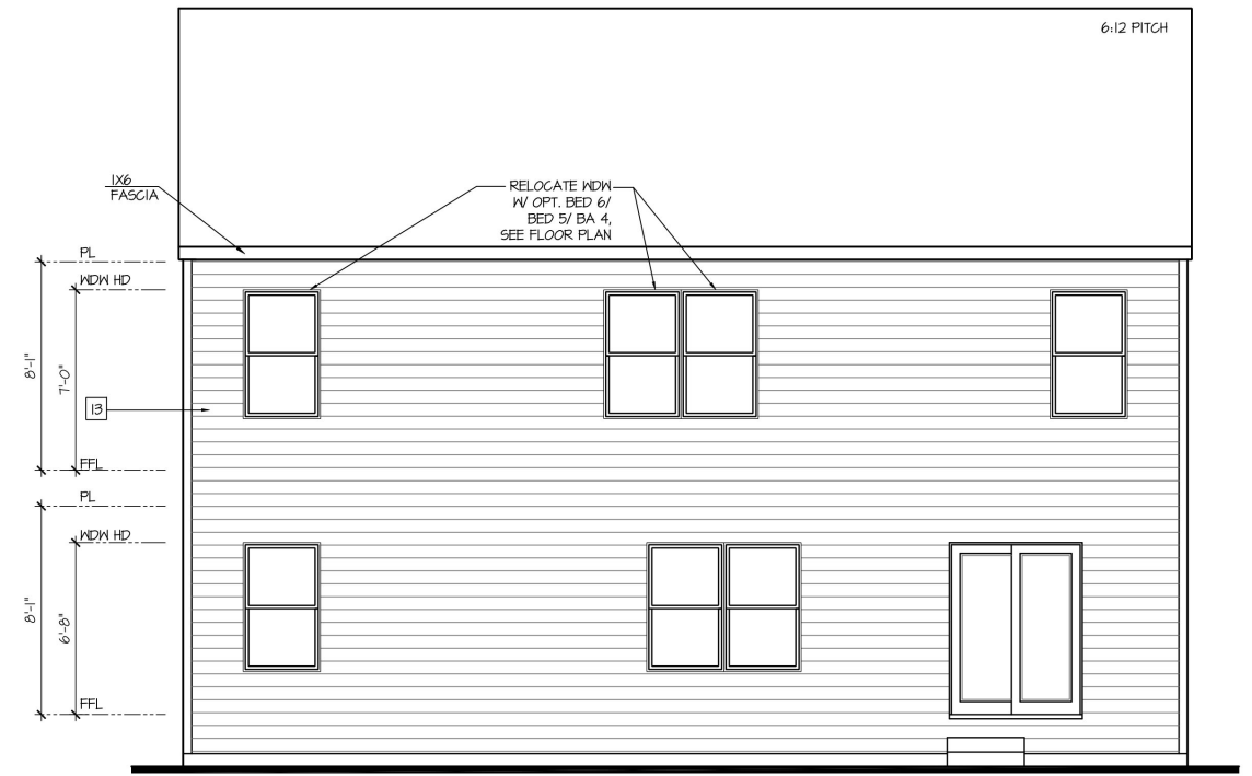
Rear Elevation 'K' w/ Opt Crawl Space SCALE: 1/4"=1'-0" AT 22'X34" LAYOUT 1/8"=1'-0" AT 11'X11" LAYOUT
