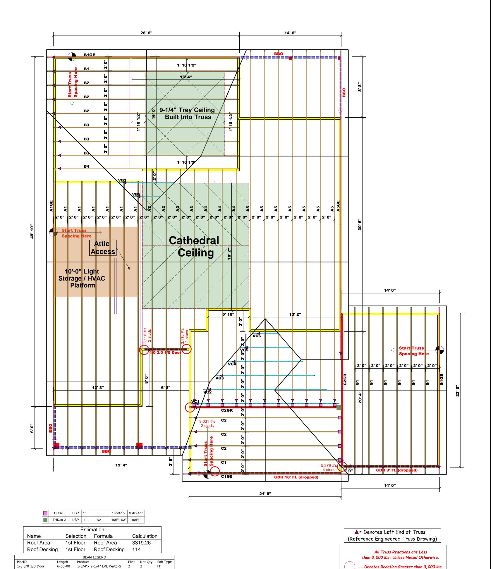
Truss Placement Plan SCALE: 1/4" = 1'-0"
