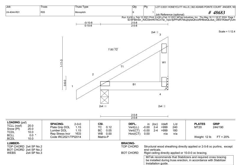
REACTIONS. (lb/size) 4=72/Mechanical, 2=162/0-3-8 (min. 0-1-8) Max Horz 2=51(LC 14) Max Uplift4=-20(LC 14), 2=-12(LC 14) Max Grav 4=97(LC 21), 2=230(LC 21)
