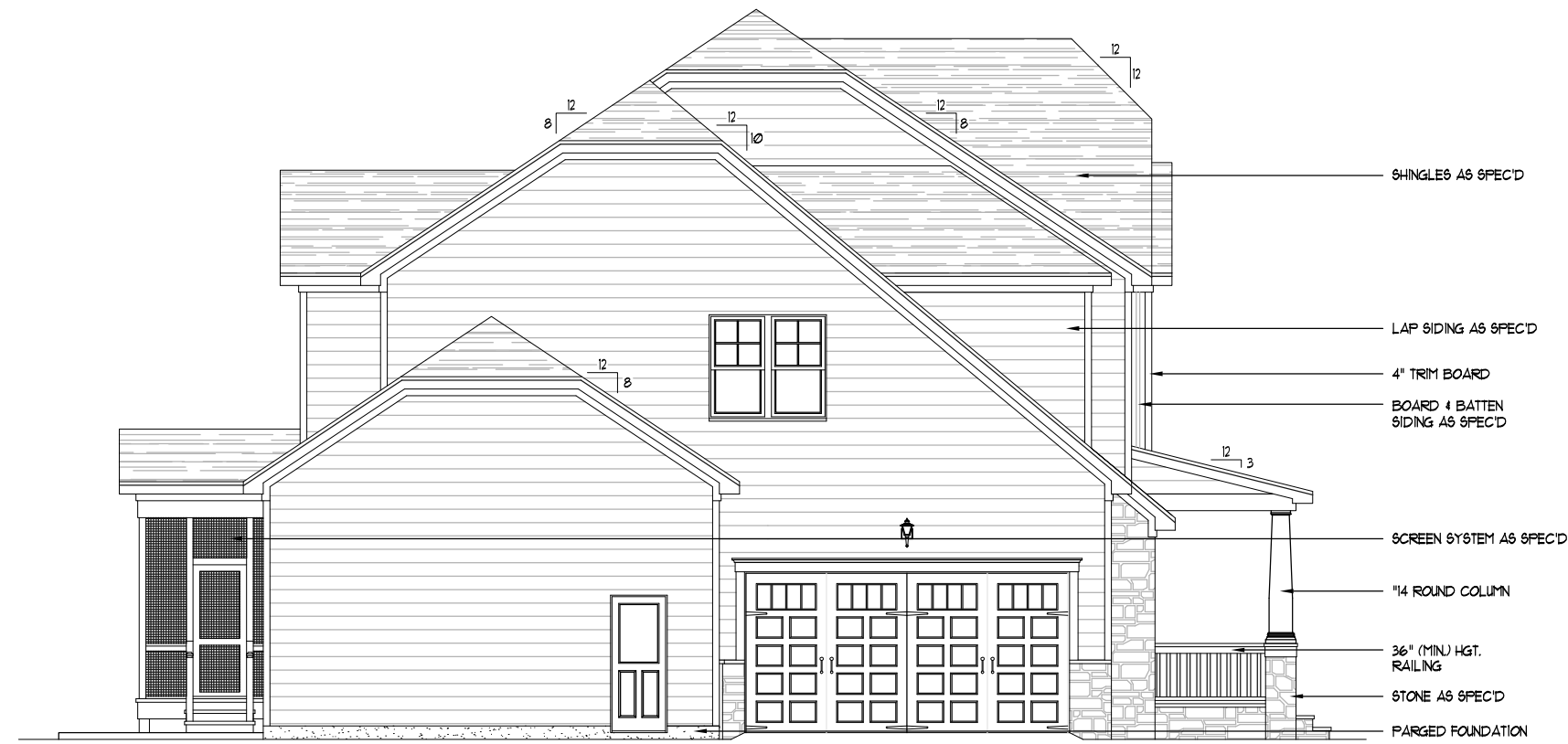
LEFT SIDE ELEVATION SCALE: ----- 1/4" = 1'-0"
