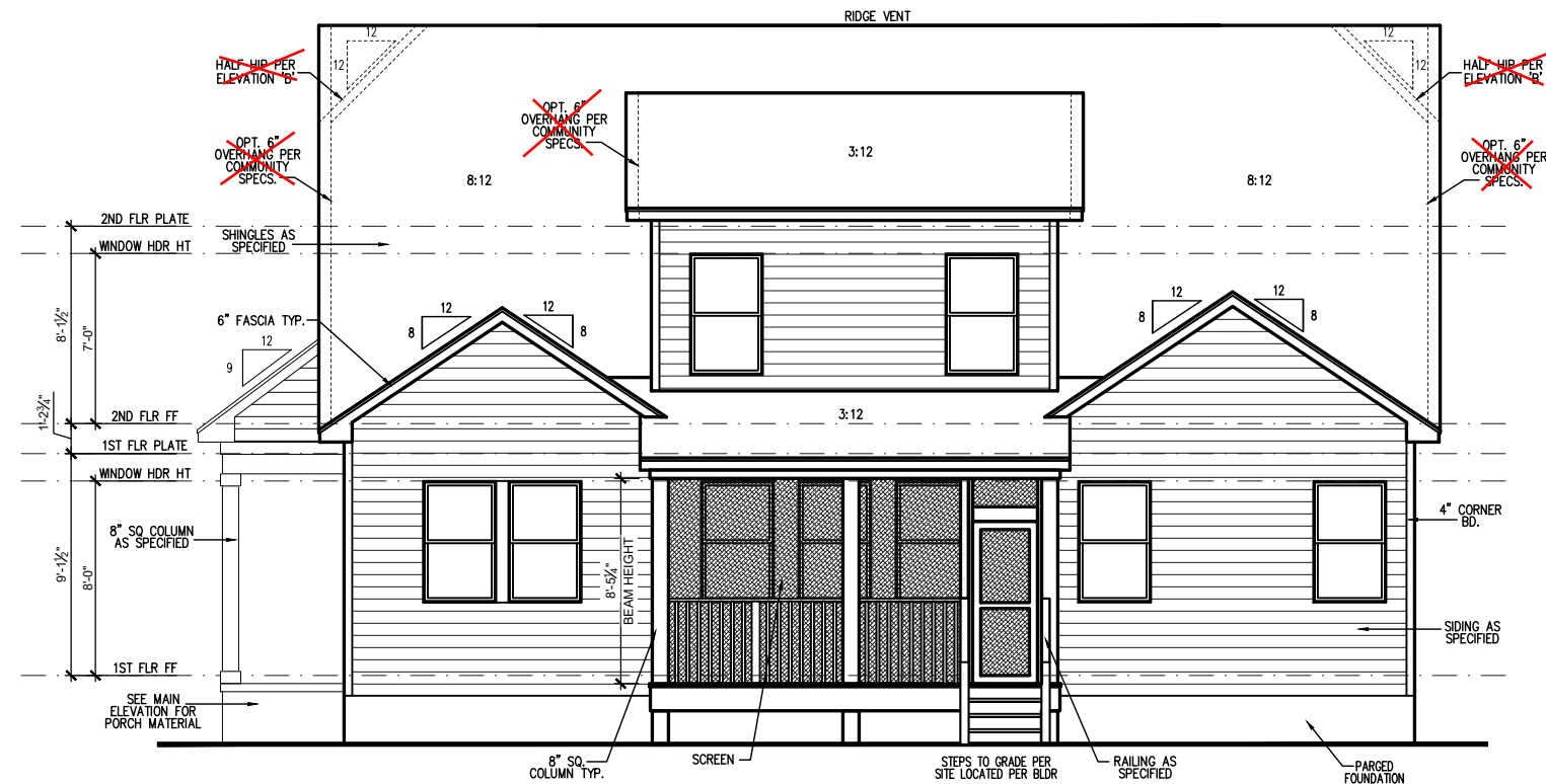
SCR. PORCH FLOOR PLAN W/ OWNER'S SUITE EXT. REAR ELEVATION SCALE: 1/8"=1'-0" ON 11x17, 1/4"=1'-0" ON 22x34
