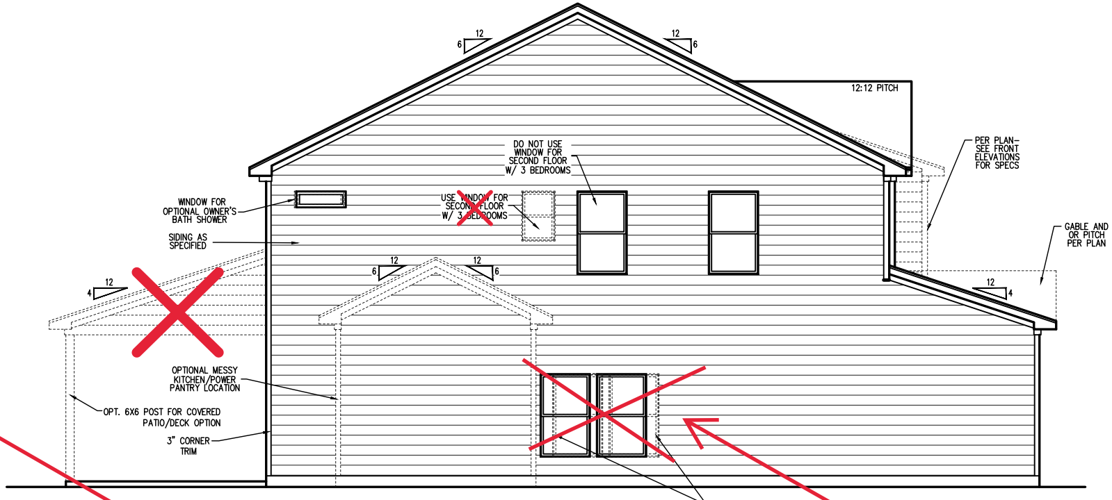
LEFT ELEVATION - (SLAB) SCALE: 1/4" = 1'-0" ON 22x34, 1/8" = 1'-0" ON 11x17
