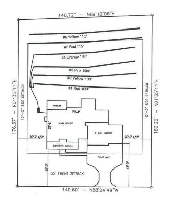
System: Gravity to serial distribution Lines: 1-4 (400') 0.3 LTAR 18" Max Trench Bottom Accepted Status System Repair: Pressure Manifold Lines: 5-6 (230') 0.35 LTAR 20" Max Trench Bottom PPBPS - 50% reduction system
