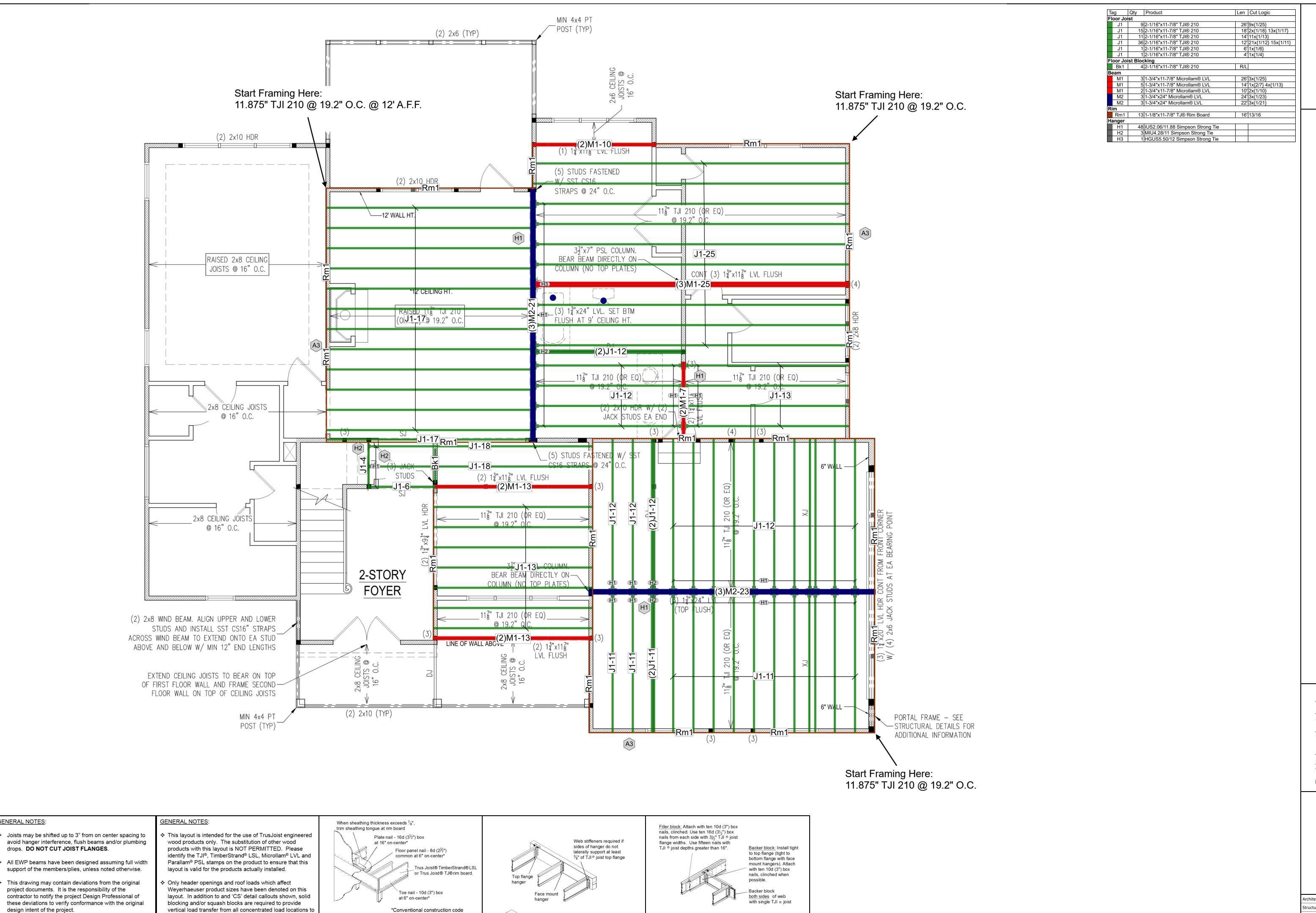
H2 With top flange hangers, backer block required only for downward loads exceeding 250 lbs or for uplift conditions.
