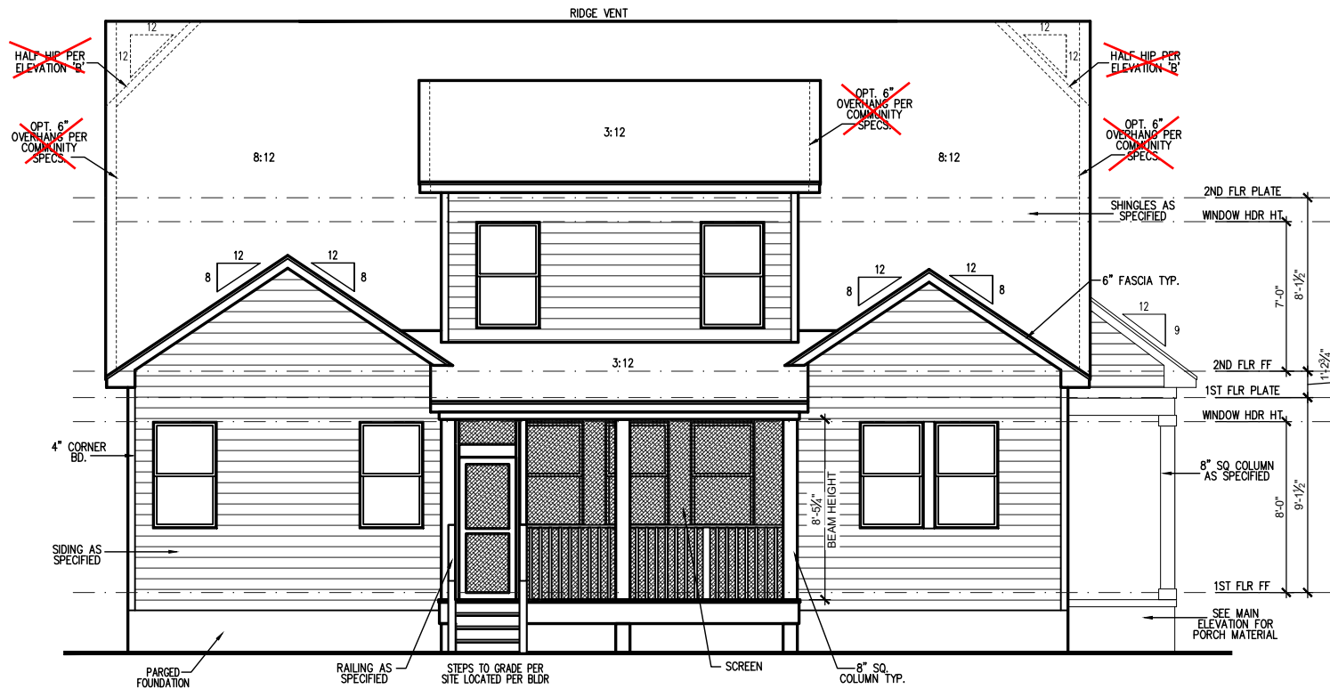
SCR. PORCH W/ OWNER'S SUITE EXT. REAR ELEVATION SCALE: 1/8"=1'-0" ON 11x17, 1/4"=1'-0" ON 22x34
