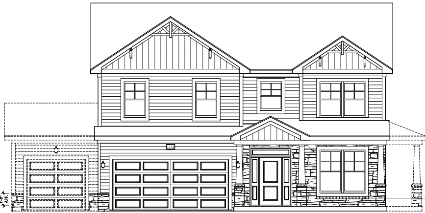
FRONT ELEVATION-B-3 SCALE 1/4" = 1'-0"
