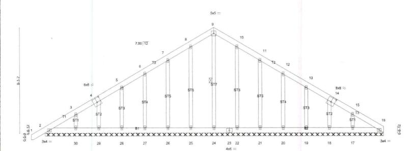
29-4-0 29-4-0 Plate Offsets (X,Y)-- [4:0-4-0,0-4-8], [14:0-4-0,0-4-8] **PLATES** GRIP LOADING (psf) SPACING-2-0-0 CSI. DEFL. I/defl L/d (loc) 244/190 Vert(LL) TCLL 20.0 Plate Grip DOL 1,15 TC 0.04 -0.00 n/r 120 MT20 TCDL 10.0 Lumber DOL 1.15 BC 0.02 Vert(CT) 0.00 n/r 120 BCLL 0.0 Rep Stress Incr YES WB 0.13 Horz(CT) 0.00 16 n/a n/a BCDL 10.0 Code IRC2015/TPI2014 Matrix-S Weight: 238 lb FT = 25%
