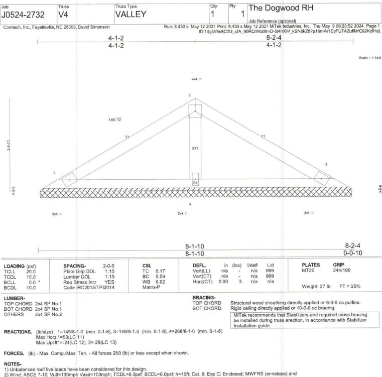
C-C Exterior(2) zone; C-C for members and forces & MWFRS for reactions shown; Lumber DOL=1.60 plate grip DOL=1.60
