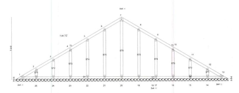
24-10-4 LOADING (psf) SPACING-2-0-0 DEFL. (loc) I/defl L/d **PLATES** GRIP TC 0.04 Vert(LL) n/a n/a 999 MT20 244/190 TCLL 20.0 Plate Grip DOL 1.15 TCDL Lumber DOL 1.15 BC 0.02 Vert(CT) n/a n/a 999 10.0 0.12 0.00 13 Rep Stress Incr YES WB Horz(CT) n/a n/a 0.0 BCLL Weight: 135 lb FT = 25% Code IRC2015/TPI2014 Matrix-S BCDL 10.0
