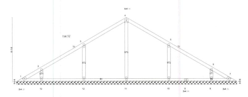
20-9-10 20-10-4 20-9-10 0-0-10 Plate Offsets (X,Y)-- [5:0-0-0,0-0-0], [6:0-0-0,0-0-0] LOADING (psf) SPACING-CSI DEFL I/defl L/d **PLATES** GRIP TCLL 20.0 Plate Grip DOL 1.15 TC 0.16 Vert(LL) n/a 999 MT20 244/190 n/a Lumber DOL TCDL BC 0.18 Vert(CT) n/a 999 10.0 1.15 n/a WB 0.10 Horz(CT) 0.00 BCLL 0.0 Rep Stress Incr YES n/a n/a Code IRC2015/TPI2014 Weight: 85 lb FT = 25%BCDL 10.0 Matrix-S BRACING-
