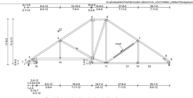
Repair for a crack in the web where indicated.
